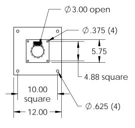
Fixed height stainless steel pedestal suited for use on IO28 and IO29 enclosure assemblies. Fully welded, sanitary design has a 1.5" NPT coupling for wiring through the pedestal assembly to the enclosure if desired.
