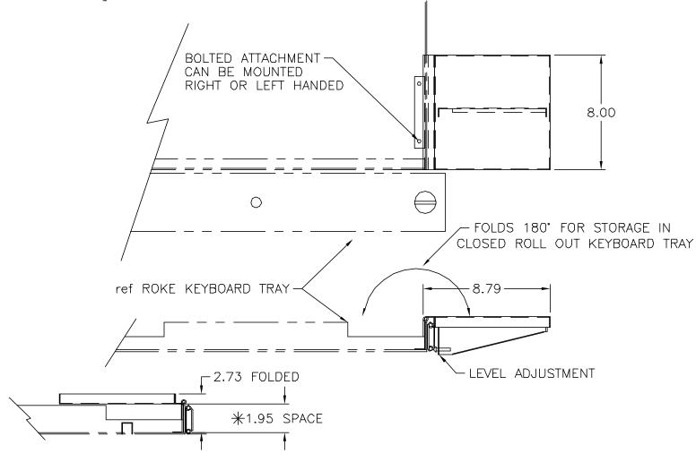
AVAILABLE SPACE FOR KEYBOARD IS REDUCED TO 1.95 INCHES LESS THICKNESS OF ANY MOUSE PAD YOU MAY ATTACH
