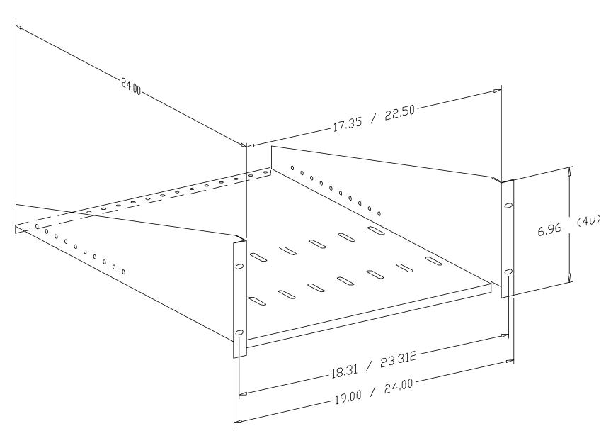
14 Ga. Steel60# Recommended CapacityBlack Polyurethane Paint
