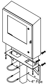
Bolt on enclosure attachment permits use of keyboard support options and openings allow cable passage.
