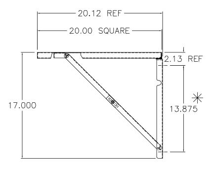
DESIGNED TO FIT IS36, IS48, IS56, IS66, IS6628 & IS6636 ICE STATIONS. MAY BE SIDE OR FRONT MOUNTED.
